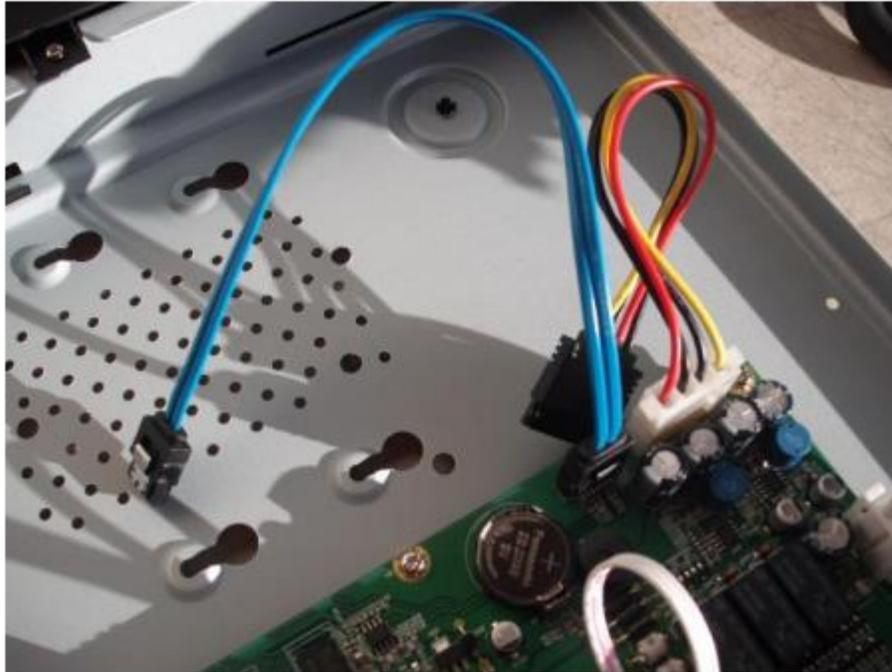
**Step 3:** Connect the other end of the SATA cable (Blue) along with the power cable (Multicolored) to the back of your Hard Drive as seen below.
