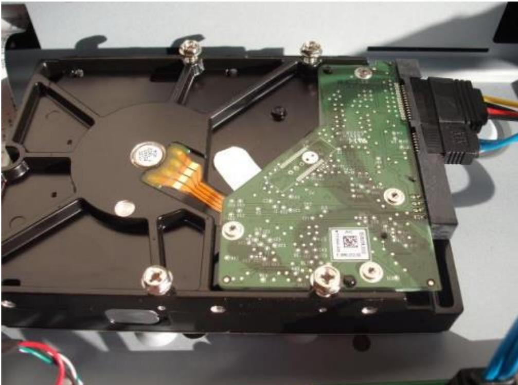
**Step 5:** Next you will need to flip the Hard Drive over and make sure the screws go into the 4 screw slots on the bottom of the DVR. Once that is complete, flip the DVR on its side, then tighten the screws to secure the HD to the bottom of the DVR.
